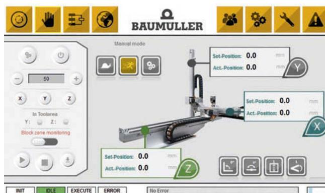
The manual mode enables the user to move to positions within a three-dimensional space. A function particularly useful when service needed.
