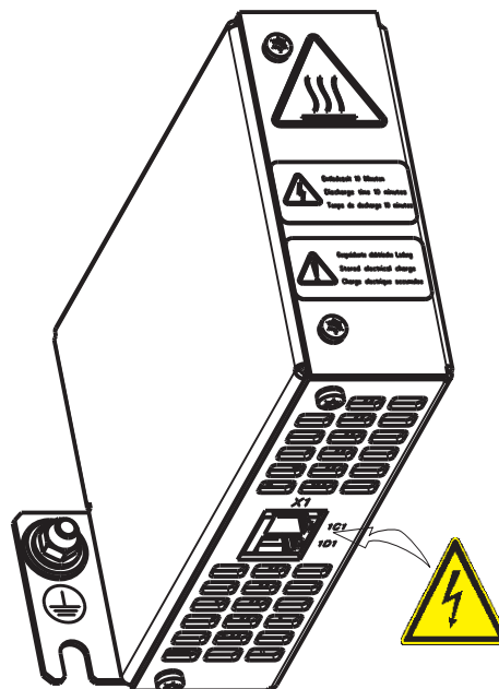
Figure 8: Hazard areas during electrical installation
