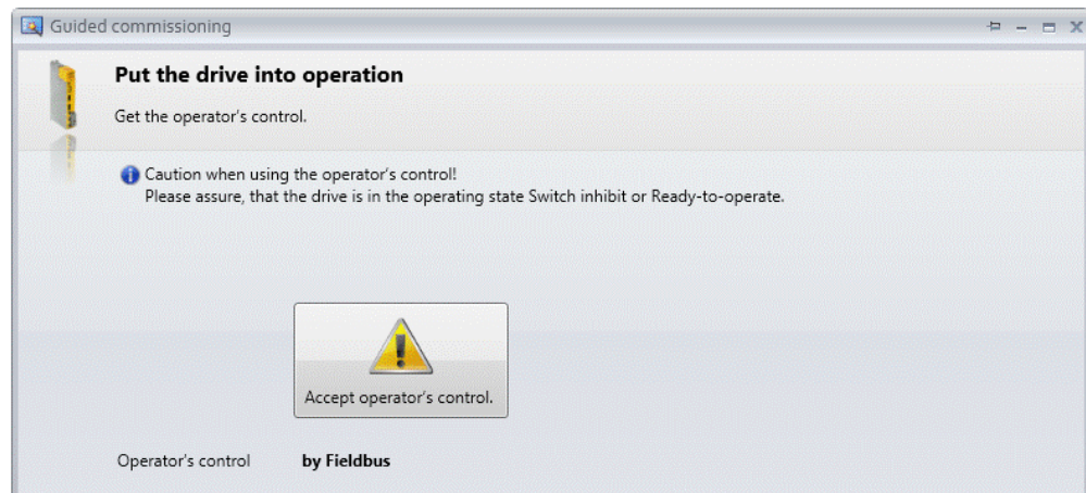
Figure 39: Guided commissioning: Operator's control
