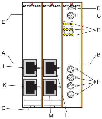
Figure 3: Module Ethernet with EtherCAT-Cluster
