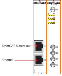
Figure 19: Connection diagram Ethernet with EtherCAT-master for b maXX controller PLC
