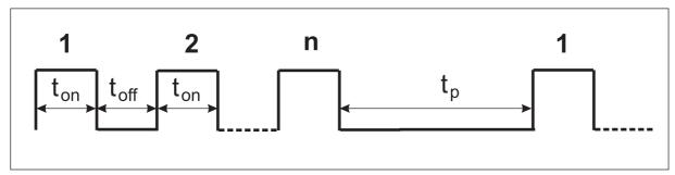
Figure 27: Blinking sequence of the LEDs
