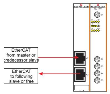
Figure 23: Example of a configuration module EtherCAT slave
