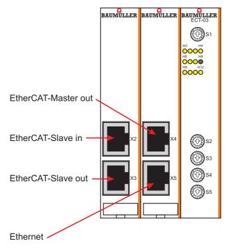
Figure 20: Connection diagram Ethernet with EtherCAT-cluster for b maXX controller PLC
