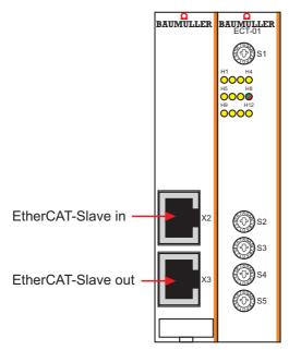
Figure 18: Connection diagram EtherCAT-Slave for b maXX controller PLC
