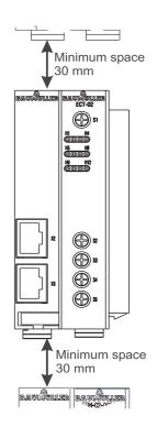
Figure 8: Installation space b maXX system
