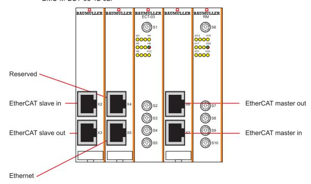
Figure 21: Connection diagram Ethernet with EtherCAT-cluster (redundant master) for b maXX controller PLC
