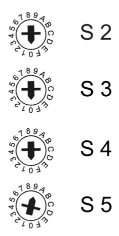
Figure 17: Example: Setting of the coding value 16H0009 (switch S2, S3 and S4 to 0, switch S5 to 9)
