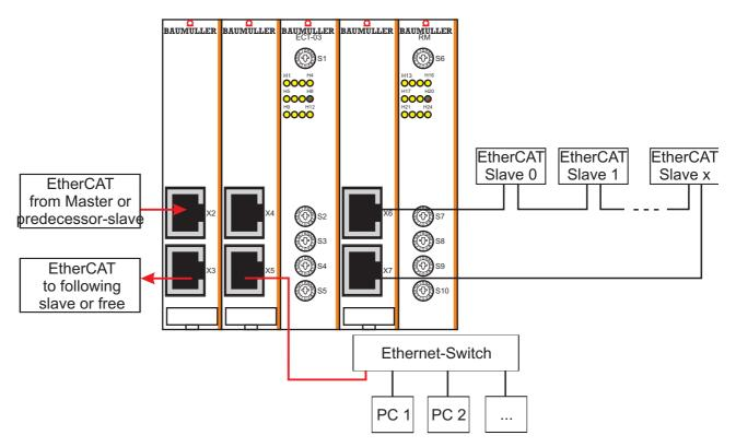
Figure 26: Example of a configuration module Ethernet with EtherCAT-Cluster with redundant master
