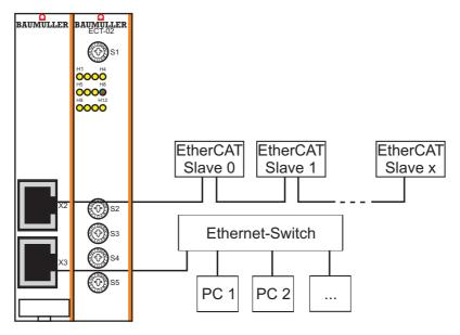
Figure 24: Example of a configuration module Ethernet with EtherCAT master
