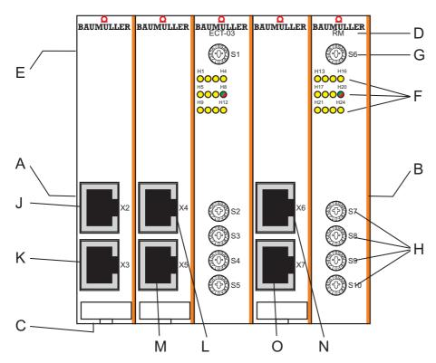
Figure 4: Module Ethernet with EtherCAT-Cluster with redundant Master
