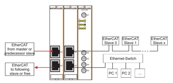
Figure 25: Example of a configuration module Ethernet with EtherCAT cluster
