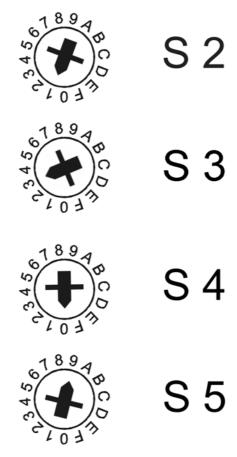
Figure 28: Example: Setting of the Ethernet-address 192.168.20.10 (switch S2 to 1, switch S3 to 3, switch S4 to 0, switch S5 to 9)
