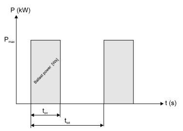
For the selection of braking resistors following formulas are valid:
