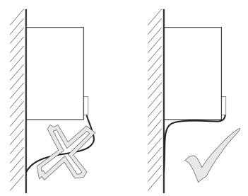
• You should route all lines as close as possible to the conductors of the ground system to reduce the effective loop area for magnetic coupling.
