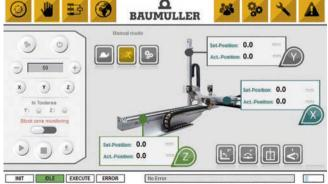
The manual mode enables the user to move to positions within a threedimensional space. A function particularly useful when service needed.
