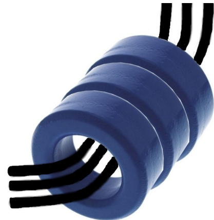
Figure 87: Mounting - several ring cores
