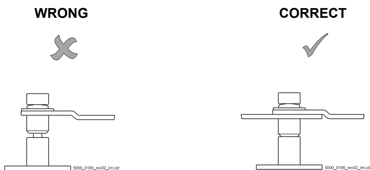
Figure 60: Mounting of the DC link bar
