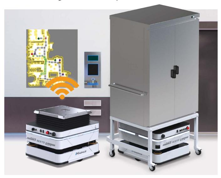
For free navigation in the room, the AMR's LIDAR sensors register the spacial situation in a teach-in run and stores this information as a map for the vehicle fleet. The map is modified using an editor integrated in the web-based interface. The positions and the "road network" are then positioned with different functions.
